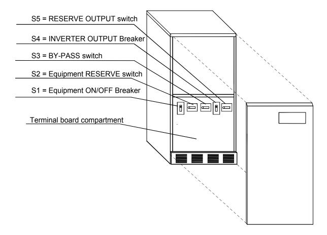
Figure 24 – 50/80kVA: Switches and Breakers
